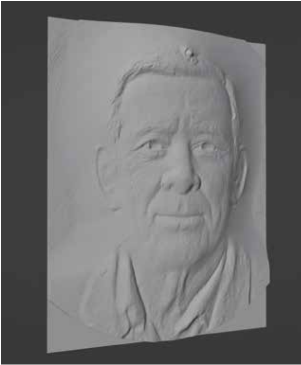
Fig 11: Miguel , automatic generation of bas-relief through photometric stereo
